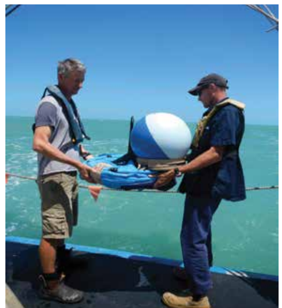
Figure 2.3 Satellite-tracked buoy being released in Australian waters aboard the Solander research vessel. Photo by Julia Reisser.
