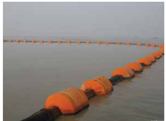
Figure 3.78 HDPE pipe with buoyancy elements
