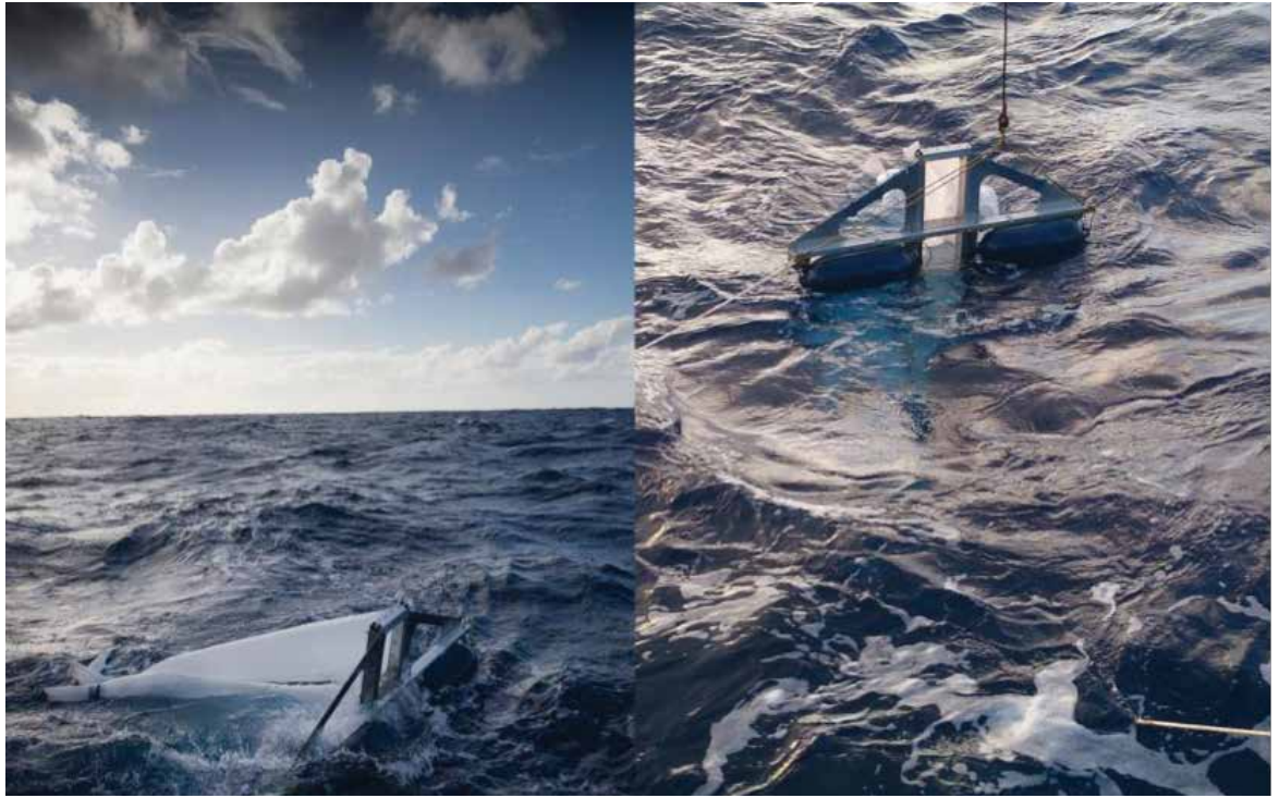
Figure 2.12 Multi-level Trawl in action during expedition 1 (left) and 2 (right). As can be seen, the trawl was higher in the water due to the angle from which it was pulled. Picture by Allard Faas
