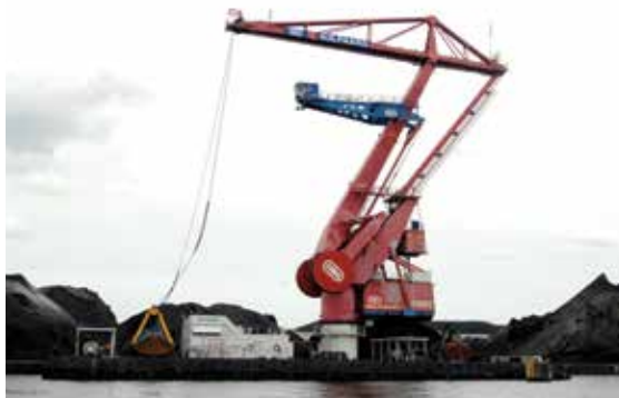
Figure 4.17 Typical grab crane. Courtesy of Pim Stouten
