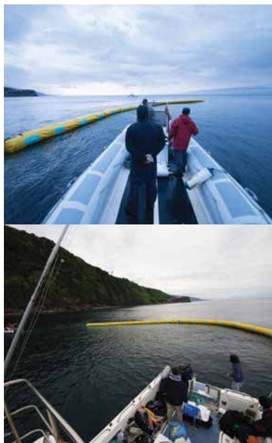
Figure 7.5 Moored barrier and pulled barrier: a) Left side, a photo of the floating barrier, moored to the seabed, b) on the right side, a photo of towing of the boom to create an artificial current using boats.
