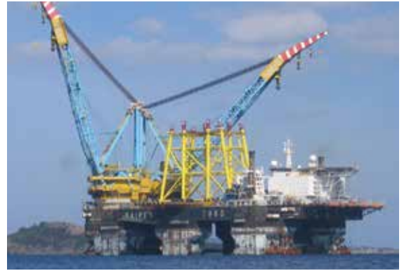
Figure 4.10 Example of a semisubmersible crane platform
