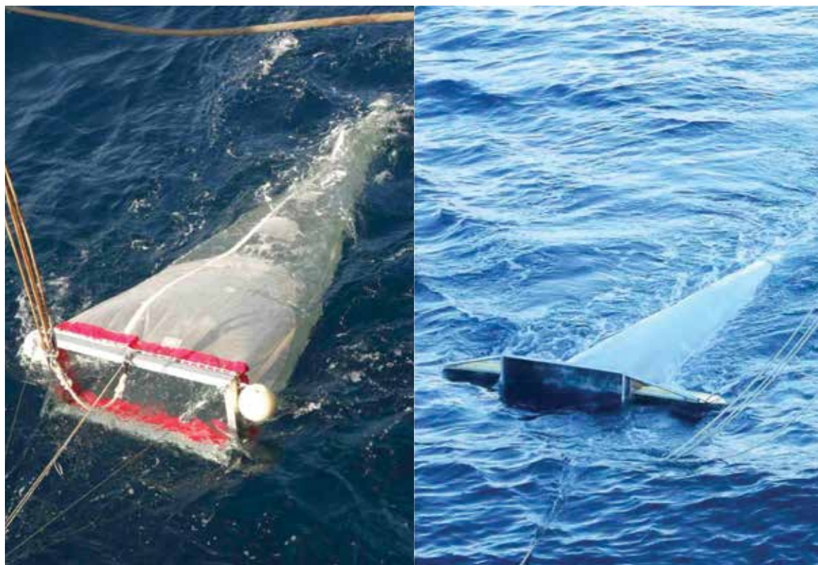
Figure 1.3 Examples of surface nets used to sample plastics at the ocean surface. Left: Neuston Net; Right: Manta Net.
