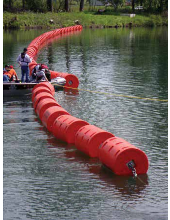
Figure 3.79 Floaters with connectable skirt
