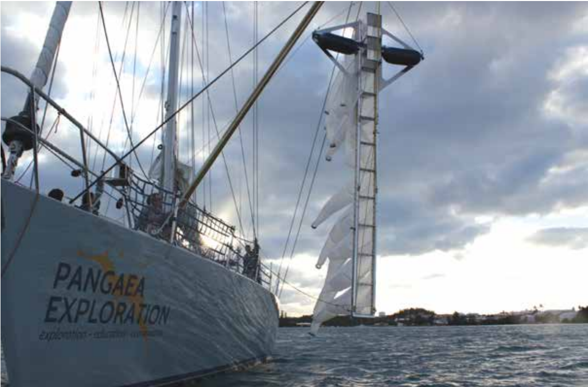
Figure 2.11 Multi-level Trawl attached to the spinnaker pole of vessel Sea Dragon, for the first expedition through the North Atlantic Gyre. Picture by Allard Faas [Figure 1b.] Courtesy of of Allard Faas. Please note that the boxes in front of the top two nets were removed after testing, and hence were not used during trawling.
