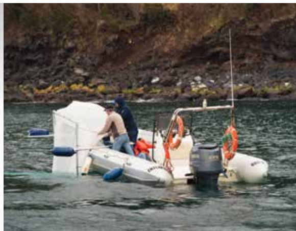
Figure 7.3 Trawl: a) Computer rendering of the trawl design, showing the metal frame, to which a net and fenders have been attached, b) deployment of trawl.
