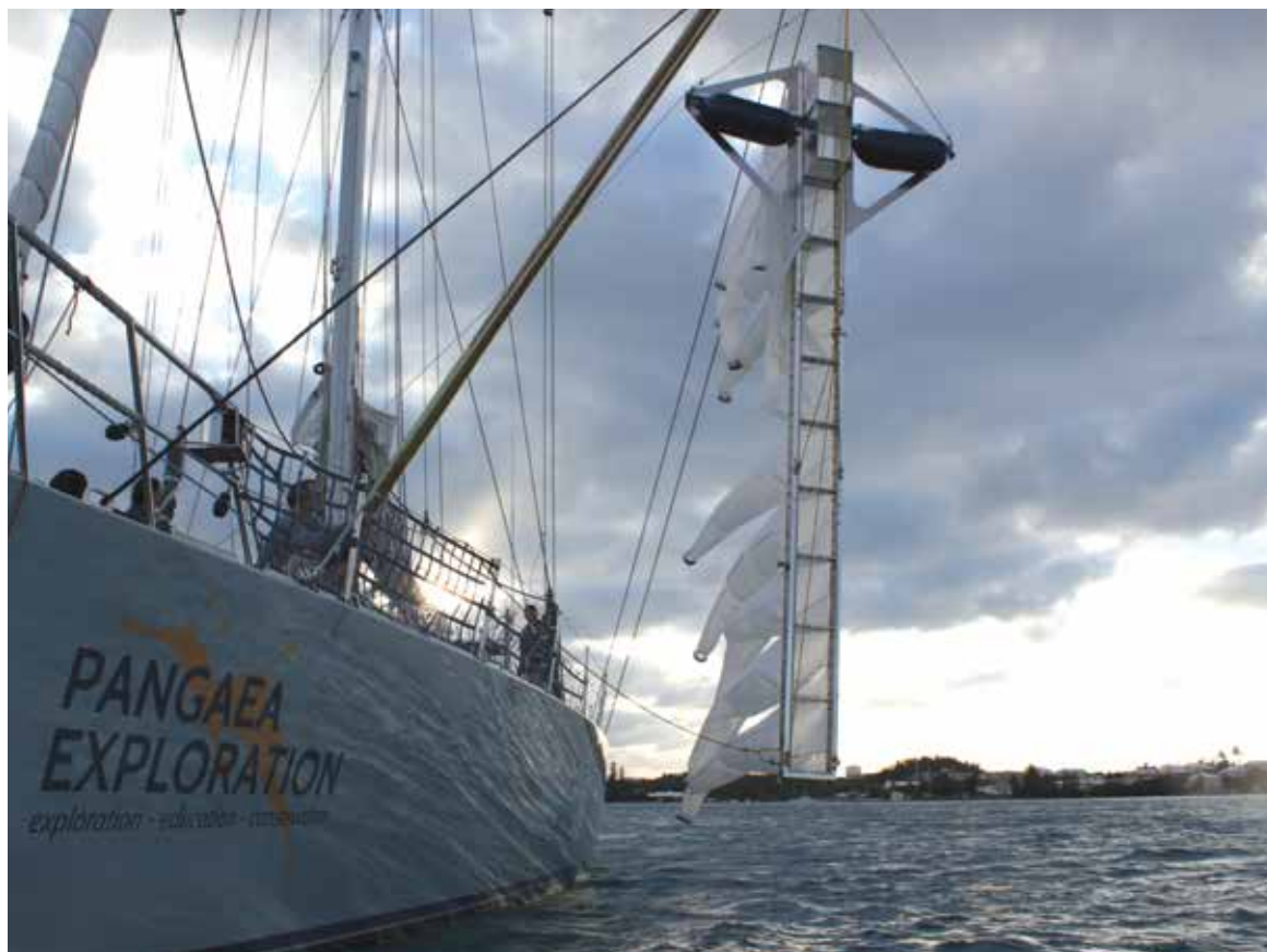
Figure 10 The multi-level trawl, used for sampling plastic concentrations
