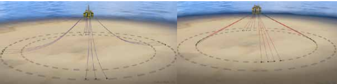
Figure 3.82 Catenary and taut leg configuration. Courtesy of C-leg media
